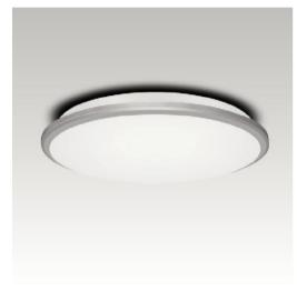
💎 1P65 🔲 🎑 SMD LM80 🦰 Material: PC Power: 30W CCT: 3000K/4000K/6500K Light source: EPISTAR SMD Light output: 2400lm Color rendering index: Ra≥80 Input voltage: AC220V-240V Driver: Built-in LED driver Operating temperature: -20°C~40°C D D  $\mathbf{E}$ (6 . . . . . Beam Angle:
